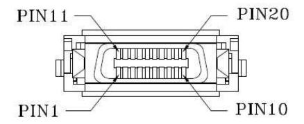
Pin-out of connector Block on Host board
