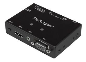
The VS221HD2VGA VGA & HDMI Auto Switch lets you connect two distinct A/V sources -- one VGA and one HDMI to the same VGA monitor or projector, and automatically or manually switch between which video source is displayed. This multi-input switch supports video resolution up to 1920x1200 (1080p) and includes mounting hardware for a tidy, professional installation.
