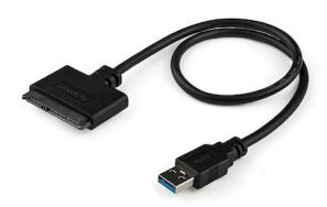
This SATA to USB cable is an external drive adapter that gives you quick and easy access to a SATA drive through the USB-A port on a laptop.
