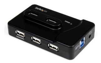
The ST7320USBC 6-Port USB 3.0/2.0 Combo Hub features a special high-output dedicated charging port which enables you to charge USB devices by providing up to 2A of power, or it can add 2x USB 3.0 and 4x USB 2.0 ports to a computer through a single USB 3.0 host connection.
