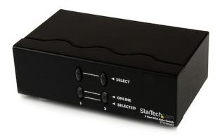
The ST122VGAU VGA Auto Switcher lets you share a display between two computers and prioritize your VGA signals. The VGA switch features a primary and secondary VGA input port, and automatically outputs the signal from the primary input. When the signal feed connected to the primary input port is cut, the switcher automatically defaults to the video signal on the secondary VGA input port.
