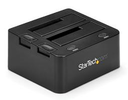
The SDOCK2U33 Dual 2.5/3.5" SATA hard drive docking station lets you dock and swap drives from your desktop or laptop computer simultaneously, using a single USB port.
