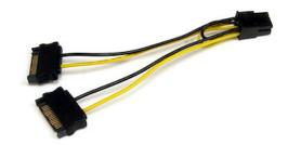
The SATPCIEXADAP SATA to PCI Express Video Card Power Adapter Cable features a 6-pin PCI Express (male) power connector as well as two 15-pin SATA (male) power connectors, providing a cost-effective way to connect a PCIe video card to Serial ATA power connectors provided by the computer power supply, and eliminating the need to upgrade the power supply for the sake of video card compatibility.
