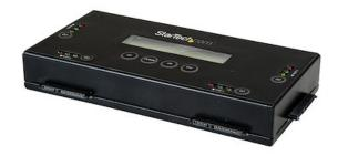
This hard drive eraser provides standalone, simultaneous drive erasing for up to four 2.5 in. or 3.5 in. SATA hard drives or solid-state drives.
