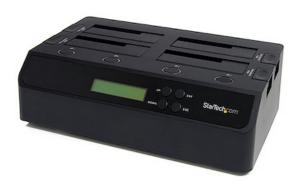
The SATDOCK4U3RE USB 3.0 and eSATA 1-to-3 Hard Drive Duplicator docking station enables you to duplicate/clone a single SATA hard drive to up to three other SATA drives simultaneously, as a standalone device. The duplicator can also function as a regular 4-bay hard drive docking station, by connecting to a host computer system. Large capacity drives (tested with up to 4TB 3.5" and 1TB 2.5" drives per bay) can be used to greatly enhance your computer's storage/backup capabilities.
