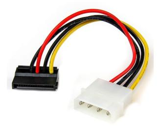
The SATAPOWADPL LP4 to 90-degree SATA power adapter features one 4-Pin LP4 male connector and a left angle, 90-degree SATA power connector (female), which enables you to power a Serial ATA hard drive from a conventional LP4 connection and eliminates the need to upgrade the computer power supply for compatibility with the SATA hard drive.
