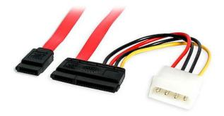
The SATA18POW SATA Data and Power Cable features a combination 22-pin SATA receptacle data and power connector as well as a LP4 power connector and SATA receptacle data connector, allowing you to create a conventional Serial ATA data connection to a computer while powering the drive through an LP4 connection to the computer power supply.
