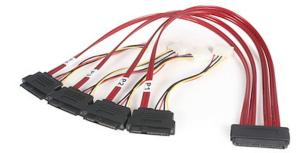
The SAS8482P50 SFF-8484 to 4x SFF-8482 SAS cable features one 32-pin SFF-8484 receptacle which fans out to four 29-pin SFF-8482 receptacles with LP4 power supply connectors, providing a reliable solution for connecting up to four SAS HDDs to a SAS controller or backplane.
