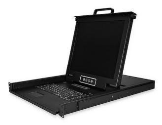
Providing centralized control of up to 16 servers, this 16-port rackmount KVM console gives you easy access to your systems. With a minimal footprint, it mounts in a server rack or cabinet using only 1U of rack space.
