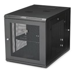
This 12U server or network rack cabinet lets you mount your EIA-310 compliant equipment to the wall, in a secure enclosure that has a hinged rear door for easy access to your equipment. The enclosure features adjustable mounting depth from 3 to 23.8 in. to provide a robust storage solution for your rack-mount equipment.
