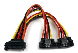
The PYO2LSATA 6" SATA Power Splitter Cable features a SATA 15-pin plug that connects to a single computer power supply SATA connector and breaks out into two latching SATA 15-pin receptacles, which enables you to connect two Serial ATA drives to a single SATA power connection on the computer power supply.
