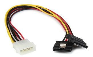
The PYO2LP4LSATA LP4 Molex to Dual Latching SATA power splitter cable features two Serial ATA female power connectors and one LP4 male connector - a reliable solution that enables you to power two SATA drives using a single LP4 connection to the computer power supply.
