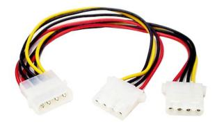
The PYO2L LP4 to 2x LP4 Power Y Splitter Cable features one LP4 male connector that breaks out into two LP4 female connectors, providing a cost-effective solution for connecting two LP4 peripheral devices (CD/DVD-ROM drives, IDE hard drives etc.) to a single LP4 connector provided by the computer power supply.
