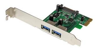
The PEXUSB3S24 2-Port PCI Express USB 3.0 Card lets you add two USB 3.0 ports to your PCI Express-enabled computer system, with an optional SATA power connector to connect to your system power supply and deliver up to 900mA of power per port to USB 3.0 bus-powered devices (500mA for USB 2.0).
