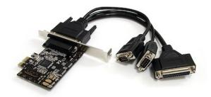
The PEX2S1P553B 2S1P PCI Express Serial Parallel Combo Card with Breakout Cable combines the functionality of Parallel and Serial cards, adding 2 RS232 serial ports and 1 parallel port through a single PCI Express (PCIe) slot.
