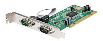
The PCI2S550 2 Port 16550 Serial Card can be installed in an available PCI slot to add two RS232 serial ports to your system. A cost-effective solution for connecting any new or legacy serial device, with data transfer rates of up to 115.2 Kbps.
