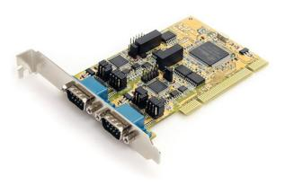
The PCI2S232485I PCI Serial Adapter Card lets you turn a PCI or PCI-X slot into 2 serial ports capable of communicating in RS-232, RS-422, or RS-485 operating modes, at baud rates up to 921.6 Kbps.
