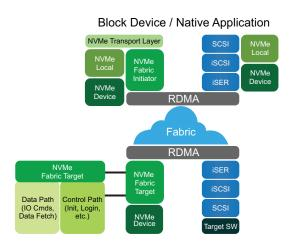
The embedded PCle switch enables customers to build standalone storage or Machine Learning appliances. As with earlier generations of ConnectX adapters, standard block and file access protocols leverage RoCE for high-performance storage access. A consolidated compute and storage network achieves significant cost-performance advantages over multi-fabric networks.
