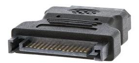
This SATA to LP4 Power Cable Adapter features one LP4 female power connector and a male SATA power connector, allowing you to connect an IDE hard drive to a Serial ATA power connector provided by the computer power supply.
