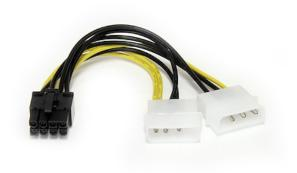
The LP4PCIEX8ADP 6-inch LP4 to 8-Pin PCI Express Power Adapter converts a standard LP4 power connector on your existing power supply to an 8-pin PCI Express video card power connector, allowing you to install a PCIe graphics card without having to upgrade the computer power supply.
