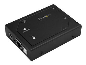
This VGA over IP extender lets you share a VGA display or projector with the wireless or wired computers on your network. The IP extender makes it easier than ever for users to collaborate and deliver presentations in boardrooms and office meetings, with intuitive controls and effortless screen sharing.
