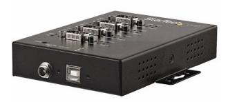
Add four extra COM ports to your laptop or desktop computer, quickly and easily. This USB to RS232/422/485 serial adapter lets you connect to your serial devices through an external USB port.
