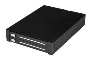
This HDD rack lets you install two 2.5" SATA hard drives or solid-state drives into a single 3.5" front bay. With configurable RAID support, the SATA drive rack provides an ideal data storage solution.
