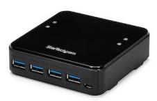
This 4 to 4 USB 3.0 peripheral sharing switch connects four USB 3.0 peripheral devices to four different computers, making it easy to switch between which computer is accessing the ports, providing a cost-effective way to create a more productive, space-efficient work area.
