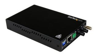
The ET90110ST2 10/100 Mbps Multimode Fiber Media Converter (ST, 2 km) lets you extend a Fast Ethernet network (10/100 Mbps) over multimode fiber, at distances of up to 2 km (1.2 miles).
