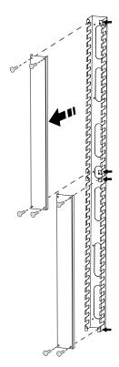
Use the ten (10) M5 x 10 screws to install the Vertical Cable Manager Body to the vertical mounting rails of your Easy Rack.
