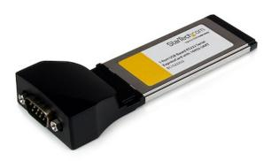
The EC1S232U2 ExpressCard RS232 Serial Adapter Card (USB-based) (16950 UART) adds an RS232 (DB9) serial port to your ExpressCard-equipped laptop, enabling you to connect an RS232 serial peripheral device such as a plotter, digital signage device, receipt printer or bar code scanner through an available ExpressCard slot.
